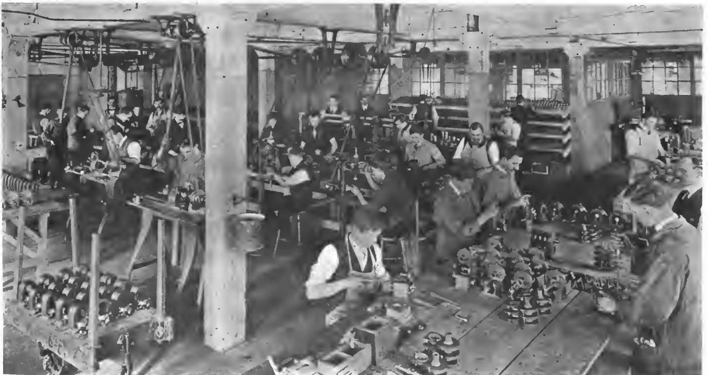
Where Splitdorf Magnetos Are Put Together With Painstaking Care That Every Part Is Right.
